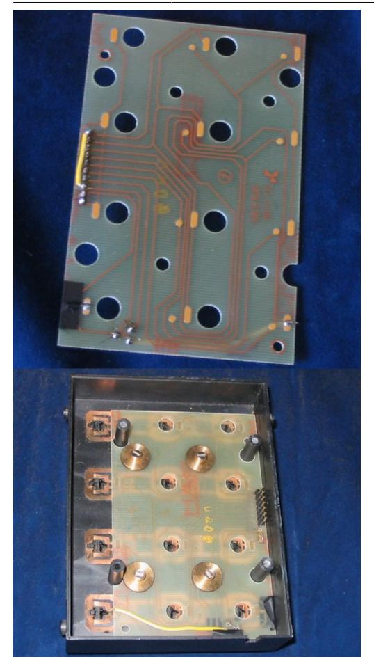
There's some space under the keypad, so I decided to mount the Core directly onto the backside of the keypad - the OPL3 module will still fit beneath it.
