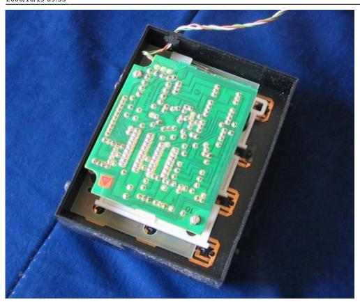
Under the control board there is a simple 4×3 button matrix (without diodes - but that's no problem, it won't be necessary to press more than one button at the same time).
