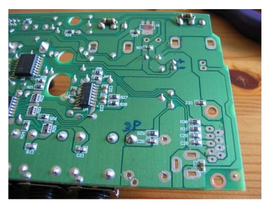
This is the lower board mounted and connected to the audio in/out jacks. Again, the capacitors are laid flat.
