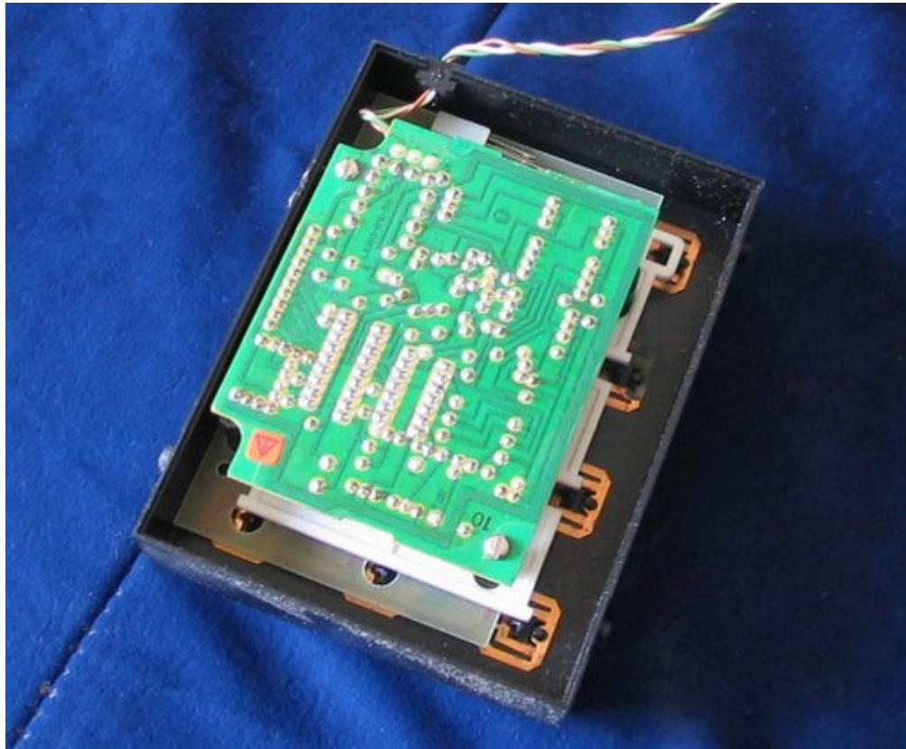
Under the control board there is a simple  $4 \times 3$  button matrix (without diodes - but that's no problem, it won't be necessary to press more than one button at the same time).
