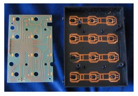
Because the contacts for the # and \* buttons were not connected, I had to solder a few thin wires and I rewired the connector:
