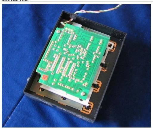
Under the control board there is a simple  $4\times3$  button matrix (without diodes - but that's no problem, it won't be necessary to press more than one button at the same time).
