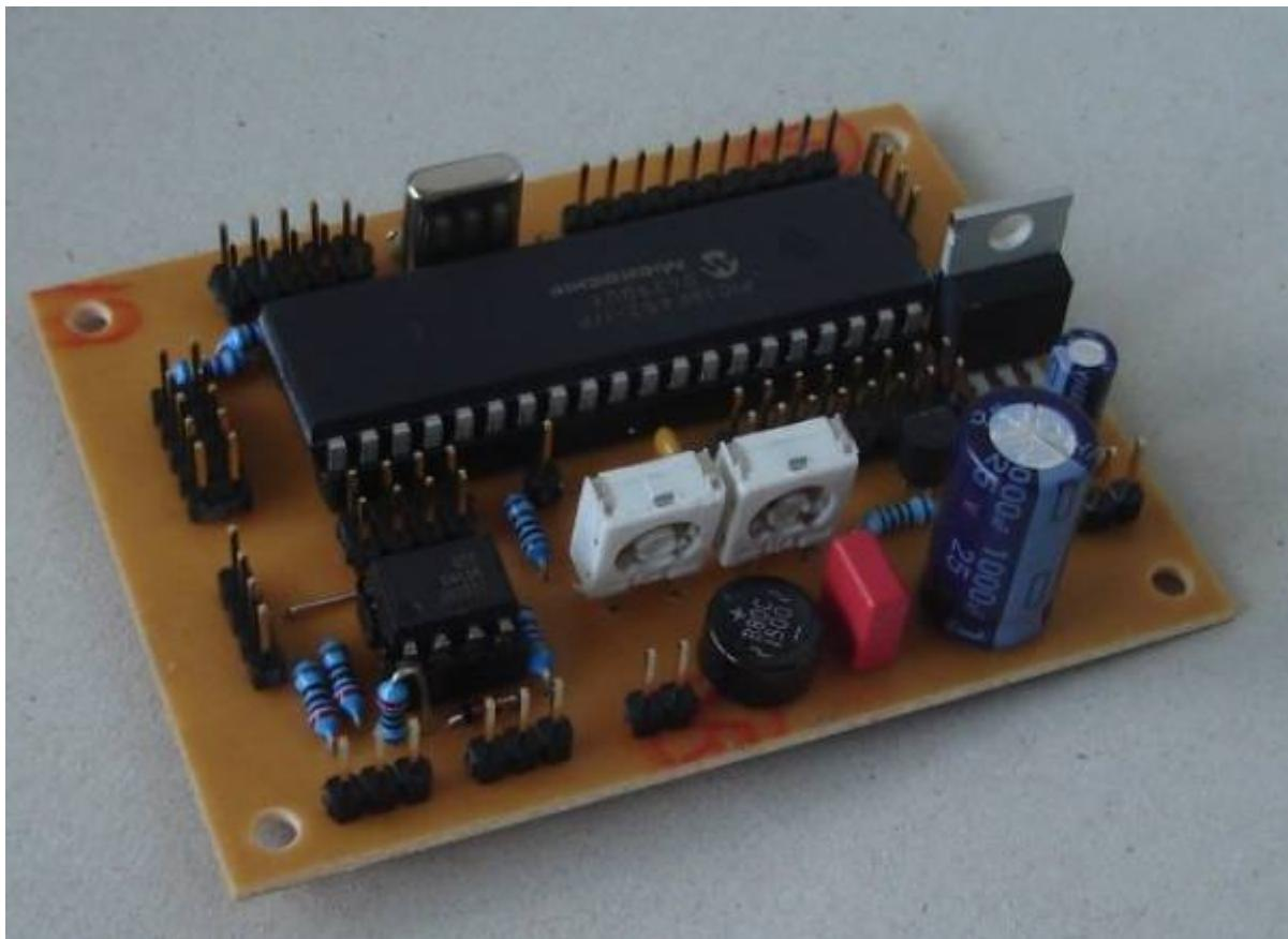
The PIC is a “**system on chip**” (**SoC**), this means, it contains not only a CPU, but also an **integrated 32k flash program memory, 1536 bytes data memory, 256 bytes data EEPROM, and a lot of usefull peripherals like AD-converter and UART (for MIDI)**. The low prices and worldwide availability for hobbyists makes it a good choice.
