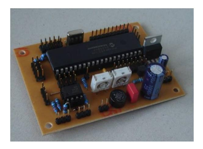
Main part of this module is the PIC18F452, a microcontroller manufactured by Microchip. It is clocked at 40 MHz (externaly with a 10 MHz crystal) and offers enough performance to handle analog and digital modules with latencies below 1ms.
