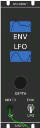
**Envelope Scope:** show the ENV-Waveform or the Mixed-CV-Output-Waveform (when Switch is in LFO Mode) and show the Envelope-Amount with a BAR or as integer Value? **MIXED CV Plug:** CV-Output > Mixed Waveform ENV+LFO
