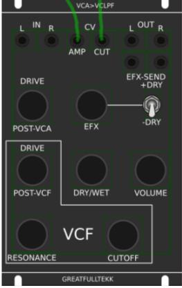
basicly a simple VCA (MS20Like) that drives the input of a Audio transformator 1:3 which is a Neutrik NTE10-3 (9€)
