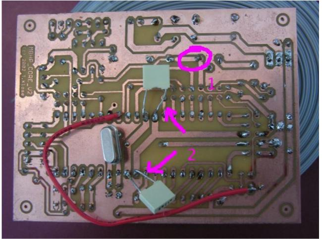
3: This seems to be a bad ground connection directly at the 78xx - it can lead to the wrong voltage. Here the same: just solder the pads again, it will help
