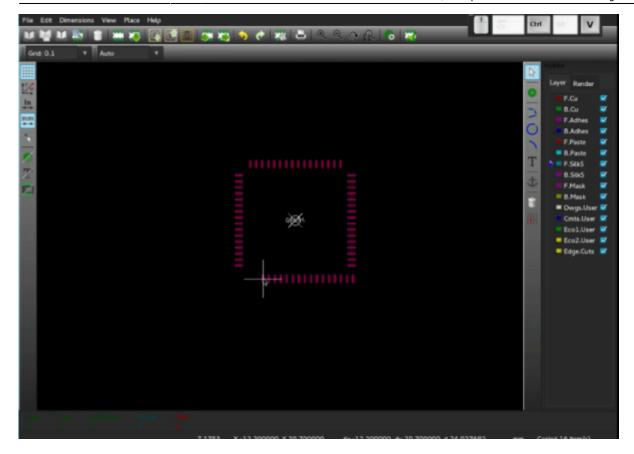
• Lastly, the PCB Design by itself. Based upon your components list and associated footprints, you can create the PCB by placing footprints at the right place and make routing between them (which is connecting components footprints by making copper paths). You can also use the famous 3D viewer to see a simulation of the result.
