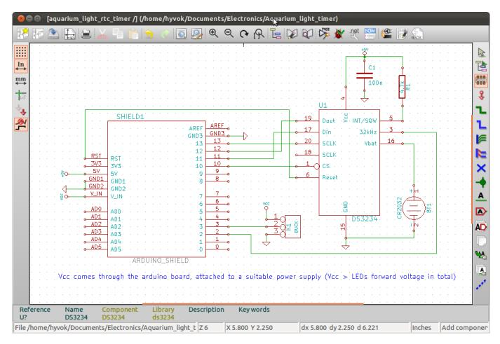
• After this you will have to make a link between components and footprints. Footprints are the layouts of pads, holes, and silkscreen drawings that are actually manufactured into the PCB, corresponding to each component.
