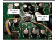
Here the signals are centered around 2.5 volts. After a few experiments I found that these signals are too weak to be fed directly into the LPCXpresso board's ADC inputs, they need some gain. The output signal of the force sensor is captured too, of course the timing requirements are much less demanding here. Here the voltage is taken directly from the force sensing resistor, just via a simple RC low pass filter to suppress noise.
