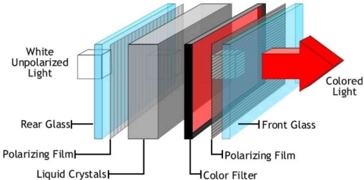
Monochrome LCD images usually appear as blue or dark gray images on top of a grayish-white background. Color LCD displays use two basic techniques for producing color, passive matrix is the less expensive of the two technologies.
