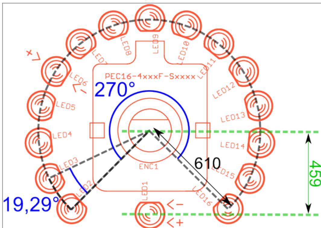
The LED polarity: the cathode (short leg) has to show to the center of the LED ring:
