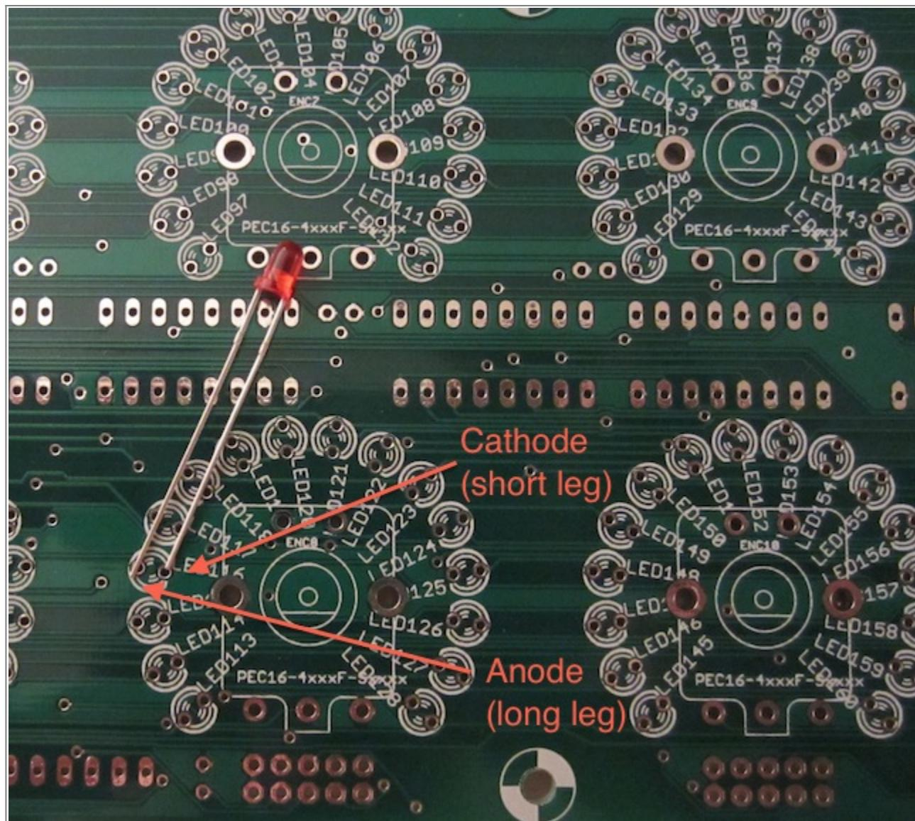
In this revision (4.6) the silkscreen of the LEDring#1 indicate the "+" (anode) and the "-" (cathode).
