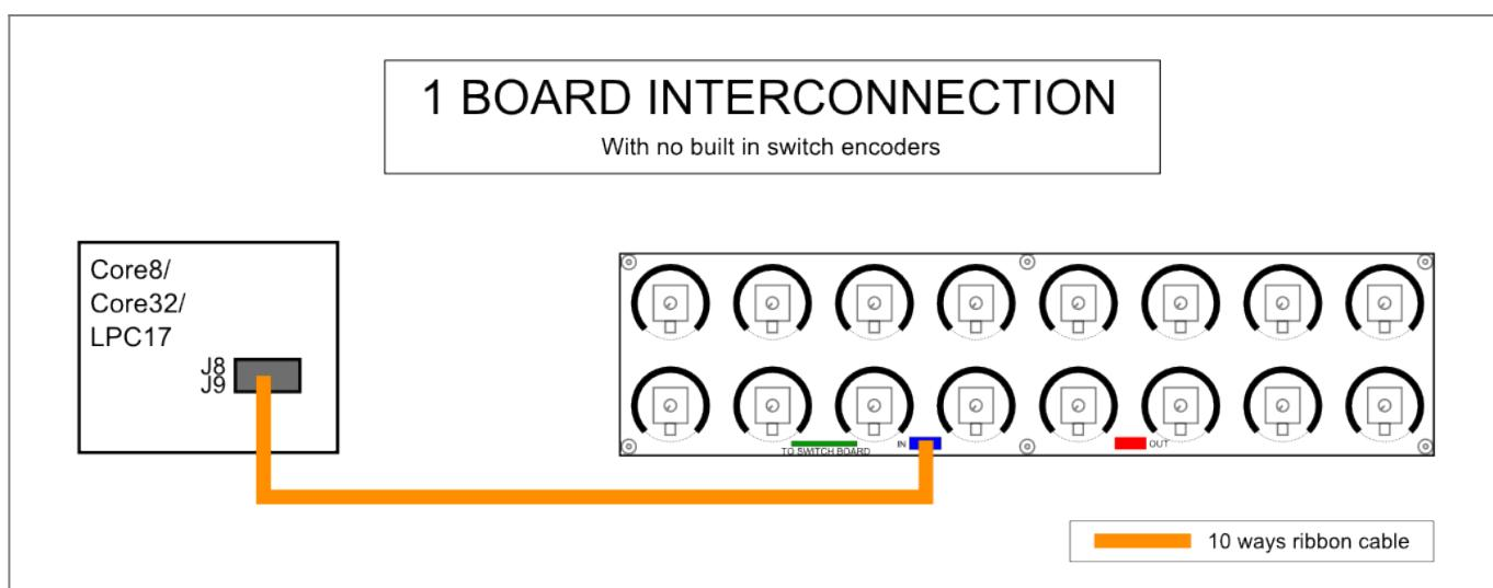
Only one 2x5 Pin IDC Ribbon Cable is necessary to connect the board.
