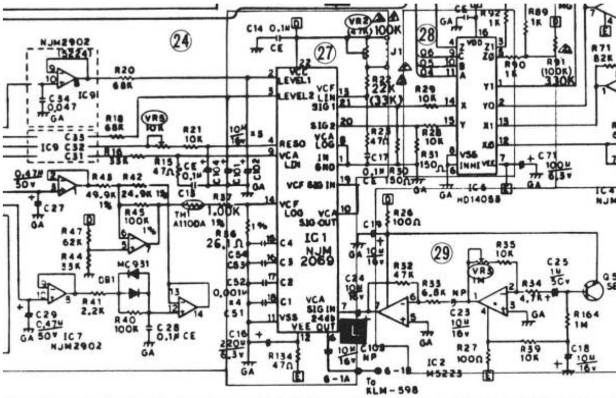
In the Poly and EX-800 the 2069 is in **PRE** configuration. It means the **VCA is before the VCF**. The VCF has 3 Voltage controlled inputs, SIG1, SIG2 and VCF In. Two VCO on SIG1 and SIG2 and a noise circuit is applied to the VCA In. The VCF 4 Poles output is the Output of the filter stage.
