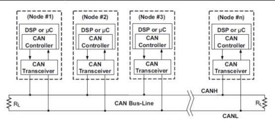
For both connection models, each Node(Device) connected to the buss can transmit or receive data. How is this possible?
