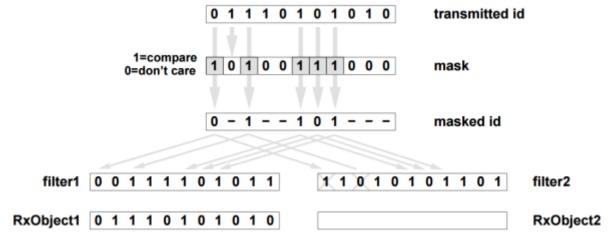
Left filter allows the packet to go into the buffer, right filter rejects it.
