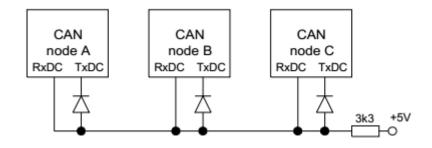
With transceivers on a 2 wire buss. All nodes are in parallel over the buss.
