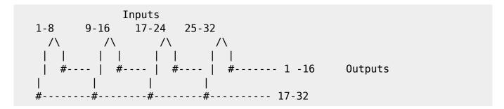
Each set of 8 inputs is split in two and goes to two chips in parallel, so that each set of 8 inputs is capable of being routed to any one of the 32 outputs, which are in two groups of 16.
