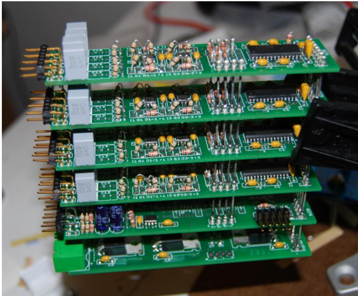
**Hardware description:** The hardware is designed in a modular form. Each mixer will need one regulator board, one output board, and some number of channel boards. All the boards are about 1" by 4", so they are quite small. They stack together to form a complete mixer. There are a LOT of choices to make before you begin to build (or even order parts). Read each of the links below to get a feel for the project requirements.
