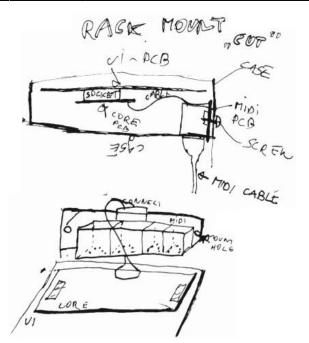
Showing a 10x4cm sized Core32 plugged into a 10x10cm UI-PCB also a midiport-solution is shown, where a midiPCB is fabricated on the core PCB but with the possibility to break it down, the optocopplers diodes and Resistors for the Midiports are on the Core PCB, so the Midi-IO pcb can be small as possibil, so we achive a small Project (small case, small ui...)
