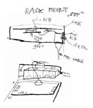
Showing a 10x4cm sized Core32 plugged into a 10x10cm UI-PCB also a midiport-solution is shown, where a midiPCB is fabricated on the core PCB but with the possibility to break it down, the optocopplers diodes and Resistors for the Midiports are on the Core PCB, so the Midi-IO pcb can be small as possibil, so we achive a small Project (small case, small ui...)
