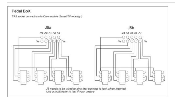
When inserting/removing a jack, make sure the control voltage = 0 (pedal off). Or you will pass voltage straight to ground, causing mios to crash, and maybe cause damage to the circuit.
