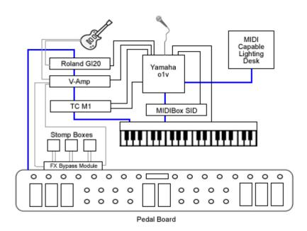
Pedal Board (and Pedal Box) can taken to the extreme. Controlling up to 7 MIDI devices. Utilising Rig Control it can set them all to your desired settings with a single stomp.
