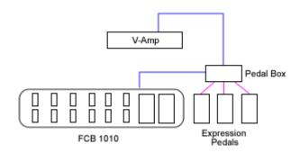
Pedal Box expands your existing floorboard with functionality very similar to Pedal Board Up to 8 Expression pedals and 8 relays can be used. Your floorboard provides the buttons.
