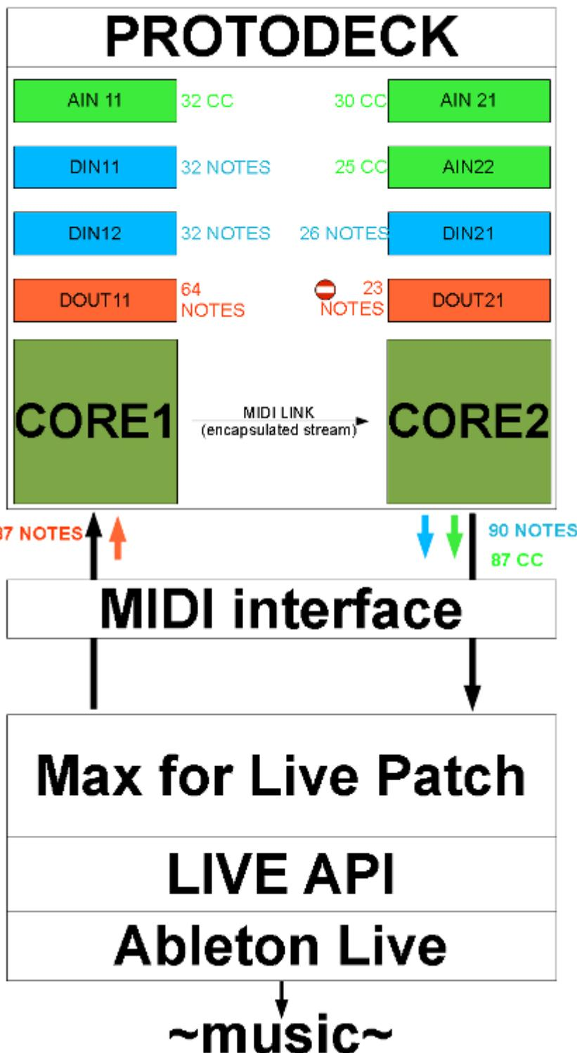
The MIDI mapping is hardcoded in the firmware in order to make it very fast.
