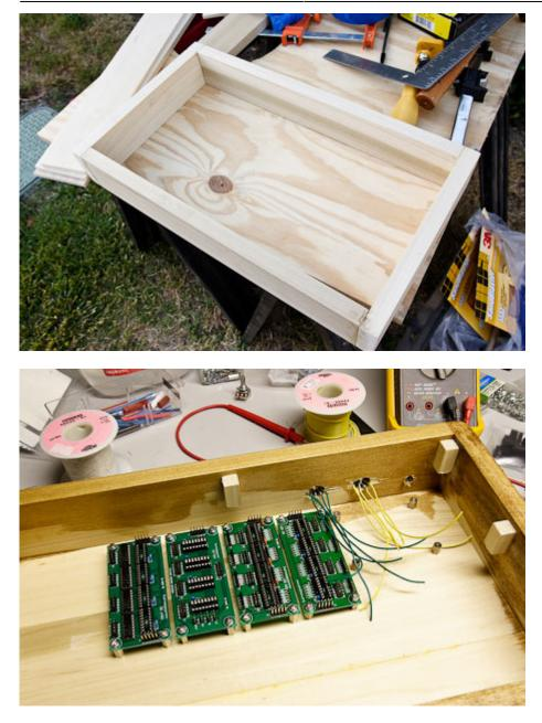
The shot above shows the module PCB's attached, awaiting the core module being hooked up to midi wiring and the power input.
