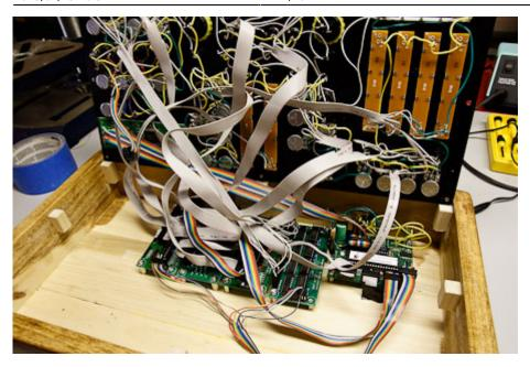
**Wiring the Panel:** Now comes the tedious and time consuming part of the build, wiring the front panel. For the most part, the PDF diagrams on the ucapps site that accompany each module are the keys to understanding the wiring sequence. I'm using ribbon cable, as it will be easy to attach to the modules, and keeps the overal spaghetti-ness of the panel down considerably.
