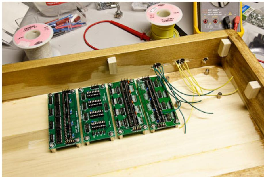
The shot above shows the module PCB's attached, awaiting the core module being hooked up to midi wiring and the power input.
