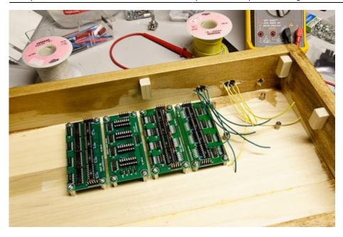
The shot above shows the module PCB's attached, awaiting the core module being hooked up to midi wiring and the power input.
