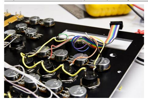
Here's a detail shot of the grounding sequence for the buttons. The black wire on the ribbon cable is connected to the VS pin on the DIN board. The rest go to their individual buttons. The black cable is then daisy-chained from one button to the next (via the yellow, thicker wire) until all of the buttons have been grounded.
