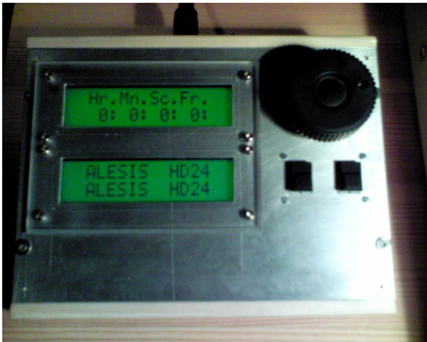
The idea with this box is to be able to do fast and precise positioning of the Alesis HD24 in combination with the LRC
