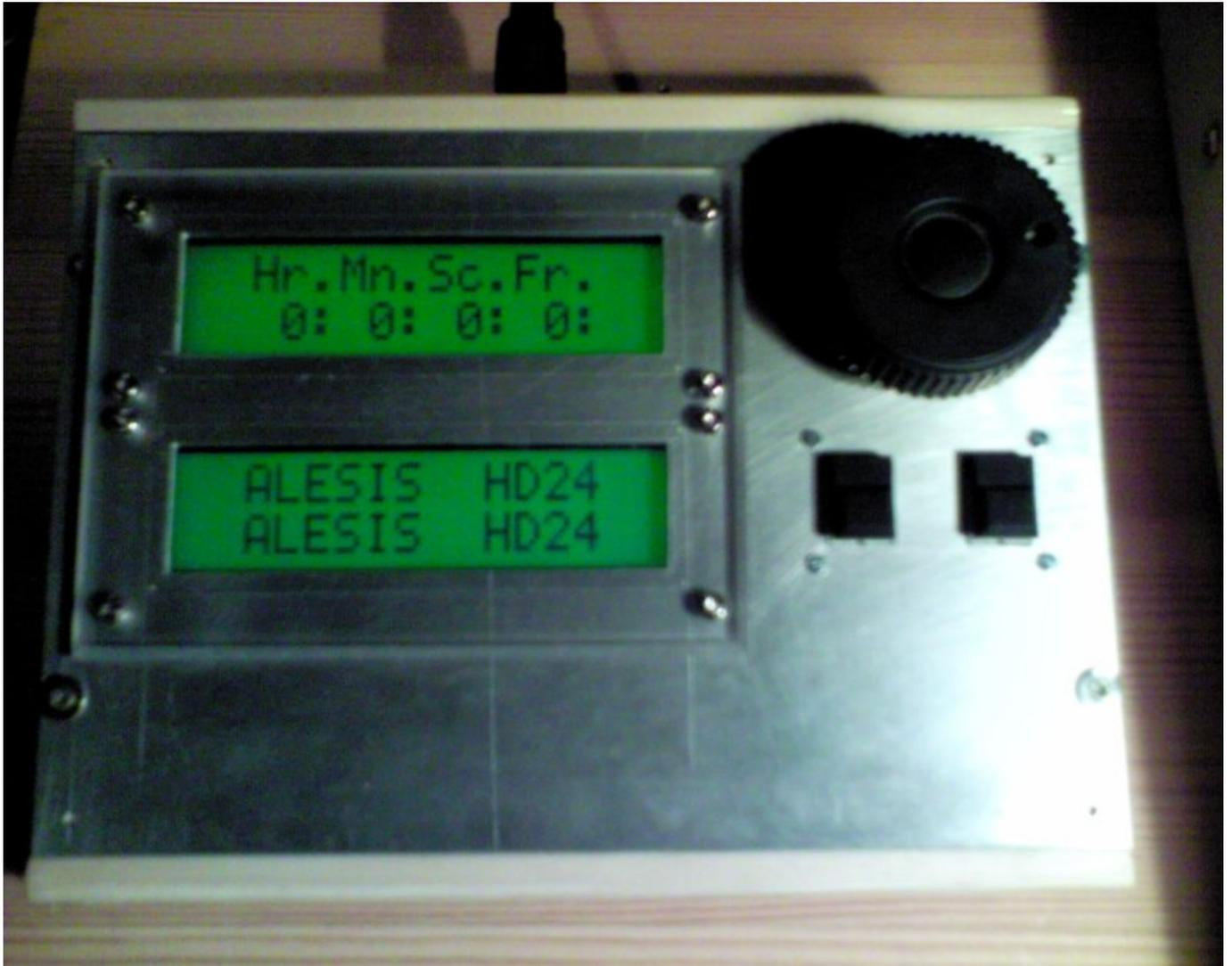
The idea with this box is to be able to do fast and precise positioning of the Alesis HD24 in combination with the LRC
