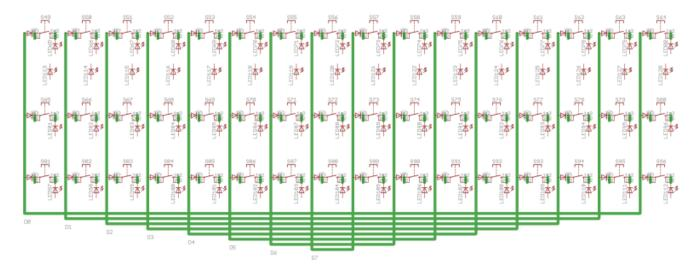
D0-D7 are used to scan switch input columns
