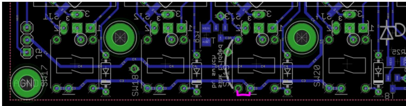
Ghosting. As seems common with these kinds of matrices, there is some unwanted lighting of LEDs. This is most apparent when trying to light up the bottom row of MEC switch LEDs, as the resistive path to the Superflux LED is lower and thus glows unintentionally. This can be overcome somewhat by stacking BAT54 Schottky diodes on top of the BC818 transistors. Later revisions will have more elegant mounting.
