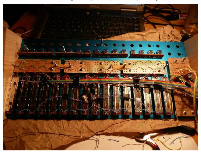
The wires were soldered directly to the module pins. This made some later de-bugging a bit painful (de-soldering, soldering, de-soldering, soldering etc.), but the connectors I used for this on the MBSeq also proved to be quite unreliable when assembly by me.
