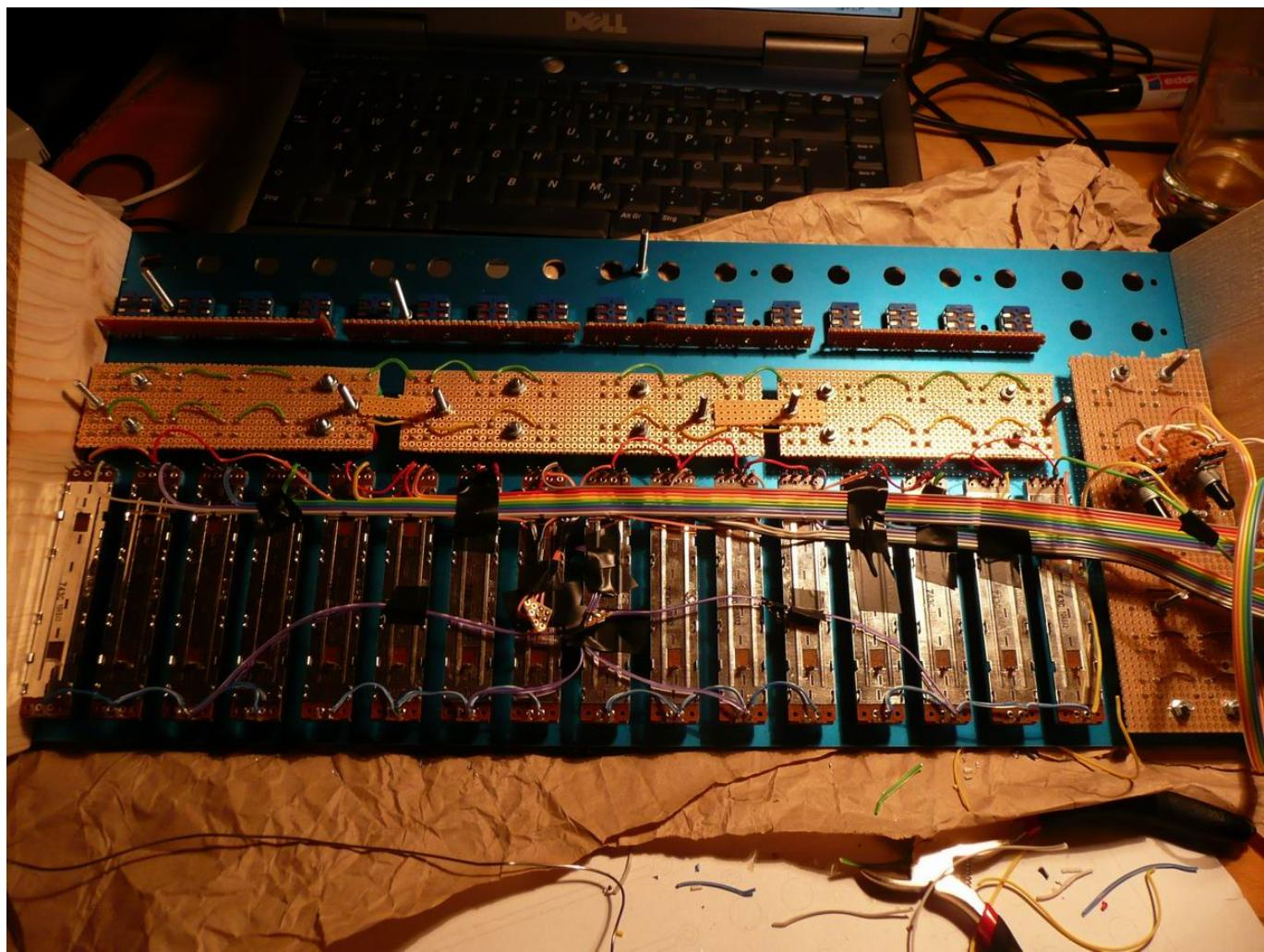
The wires were soldered directly to the module pins. This made some later de-bugging a bit painful (de-soldering, soldering, de-soldering, soldering etc.), but the connectors I used for this on the MBSeq also proved to be quite unreliable when assembly by me.
