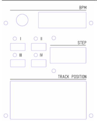
The cutouts for the 7-segment displays and the LED matrix modules hold little plexiglass windows that I had also made at Ponoko. I have access to a (manual) milling machine, so I milled a groove surrounding each cutout on the backside of the panel. The plexiglass window has an identical groove on the front so that the two sit flush and can be glued together quite easily. You probably don't need the two inner mounting holes (above and below the STEP display) at all.
