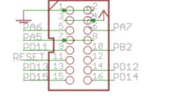
The original J16 functionality is preserved, but extra pins are available on an IDC16 header. These include the Reset signal and pins normally controlling LEDs. This header is normally connected to the RES-SD module.
