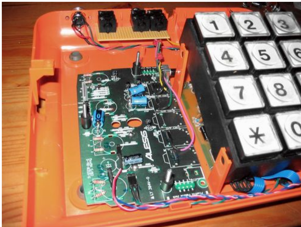
The second board connected. Behind the keypad there's the Siblance pot.
