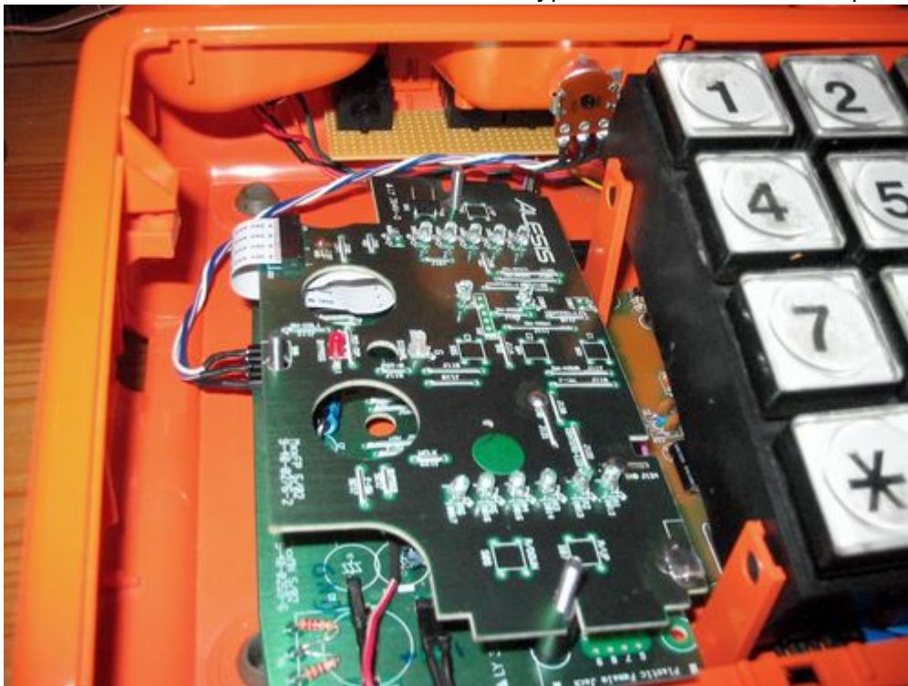
The pot and jacks seen from behind:
