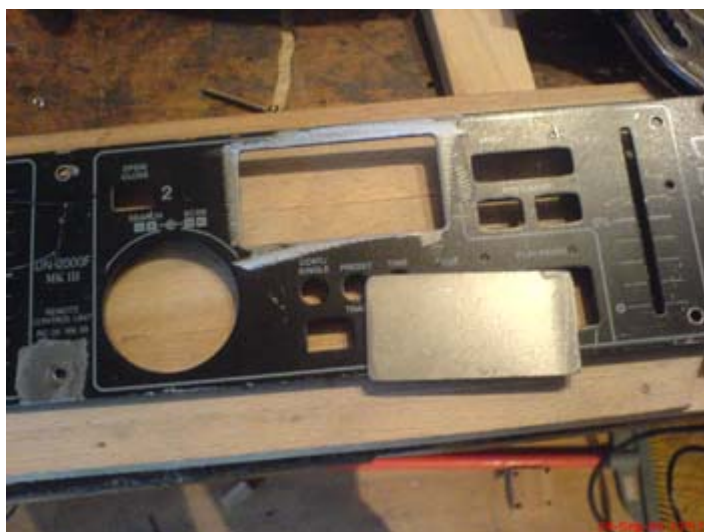
Partly finished after bondding and sanding.
